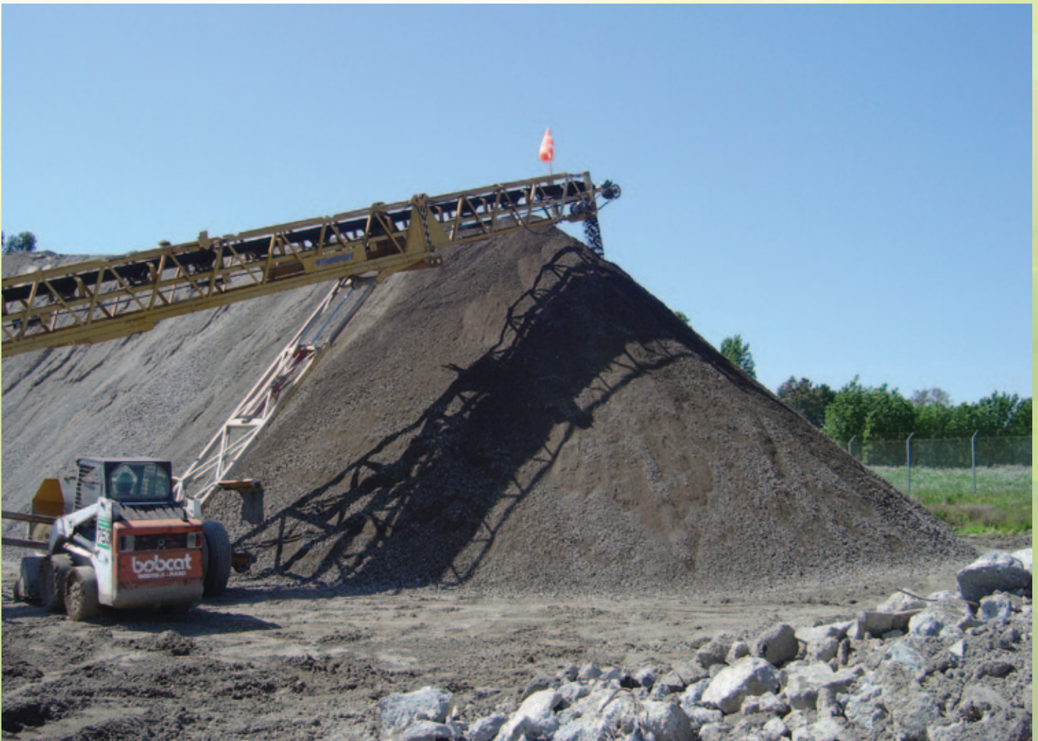
OAK: Stockpiled Asphalt, Concrete, and Soil Blended to Create Material for Airport Pavement
